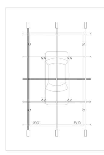
The lighting is installed on a freestanding, wide-span structure comprising lattice beams with integral tracks. Spotlights and projectors are used for striking accent lighting and clearly defined beams and gobo projections.
